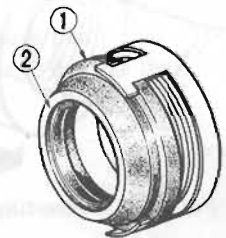
Fig. AC-83 Checking shaft seal
