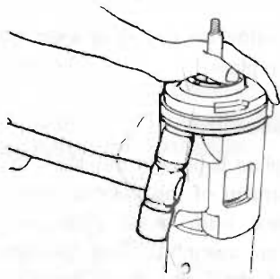
Fig. AC-100 Removing front end cover
