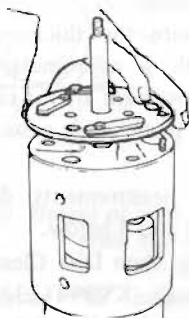
Fig. AC-102 Installing cylinder head
